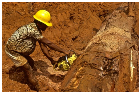
Above: Heavy work in mud 'bucking' this log. Bare feet is the best thing under such conditions.
