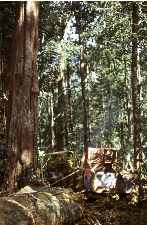
A large dun ( Doona zeylandica ) log being hauled out by a Timberjack 404 skidder, assisted by a D6 Caterpillar.
