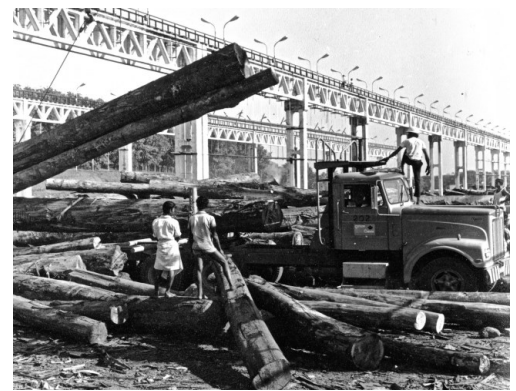
Unloading one of the Hayes trucks at the Kosgama wood yard using an overhead crane. On days when the cranes were broken down, individual logs had to be hitched to a sturdy post and the truck driven forward, thus randomly dumping the load. It was a scene of general chaos.
